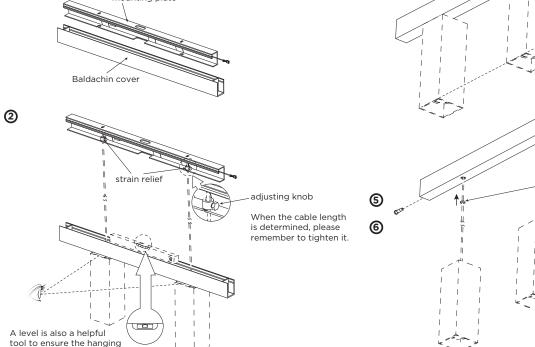
MOUNTING INSTRUCTION Remove the mounting plate from the baldachin cover.
